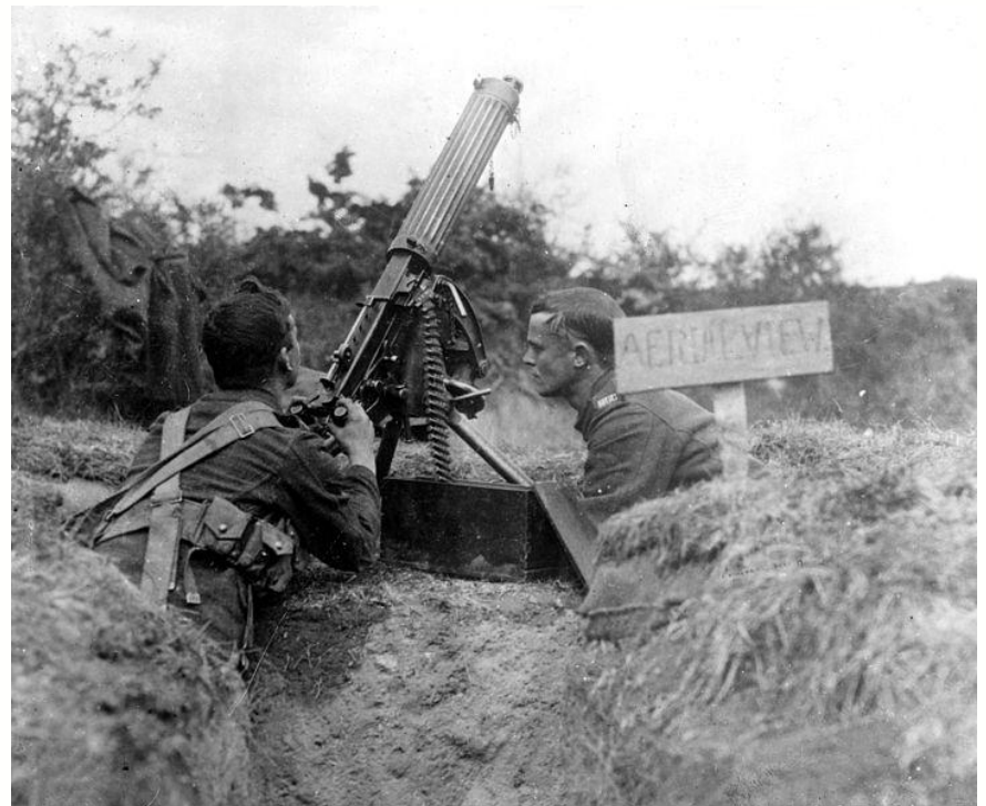
British Vickers machine gun, shown set up for anti-aircraft purposes. Photographed circa 1914-1918. (Wikimedia Commons)
