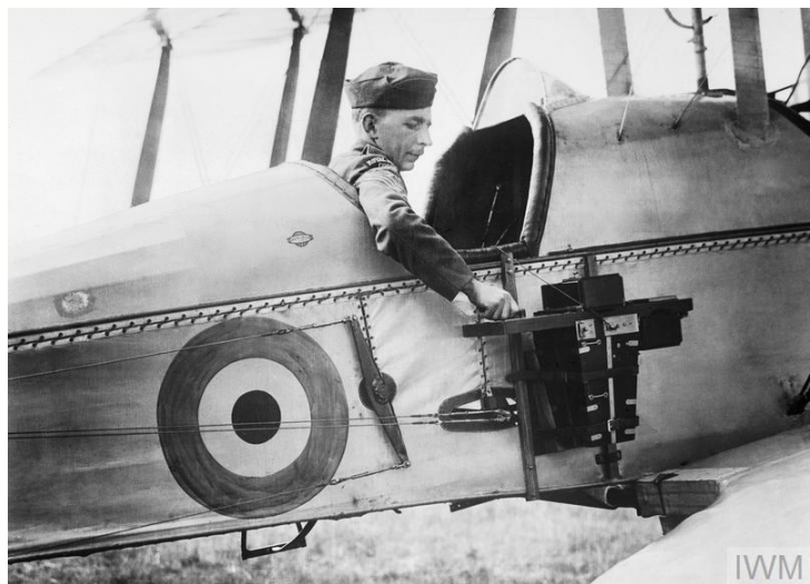
A sergeant of the Royal Flying Corps demonstrates an aerial reconnaissance camera fixed to the fuselage of a BE2c aircraft, 1916. © IWM (Q 33850)
